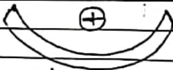
Sagging curve positive Bending moment
