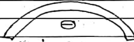
Hogging curve Negative Bending Moment
